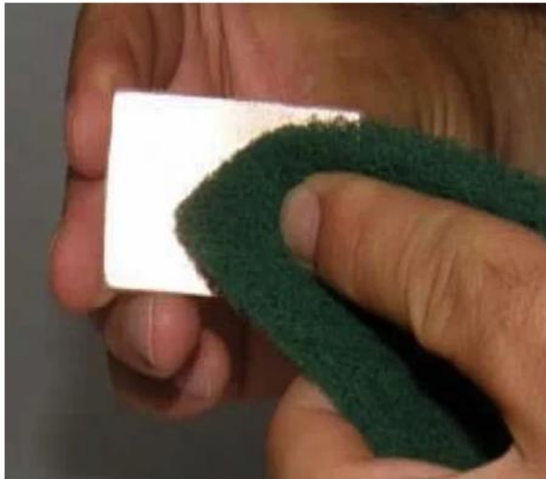
Rubbing away the top oxide layer
